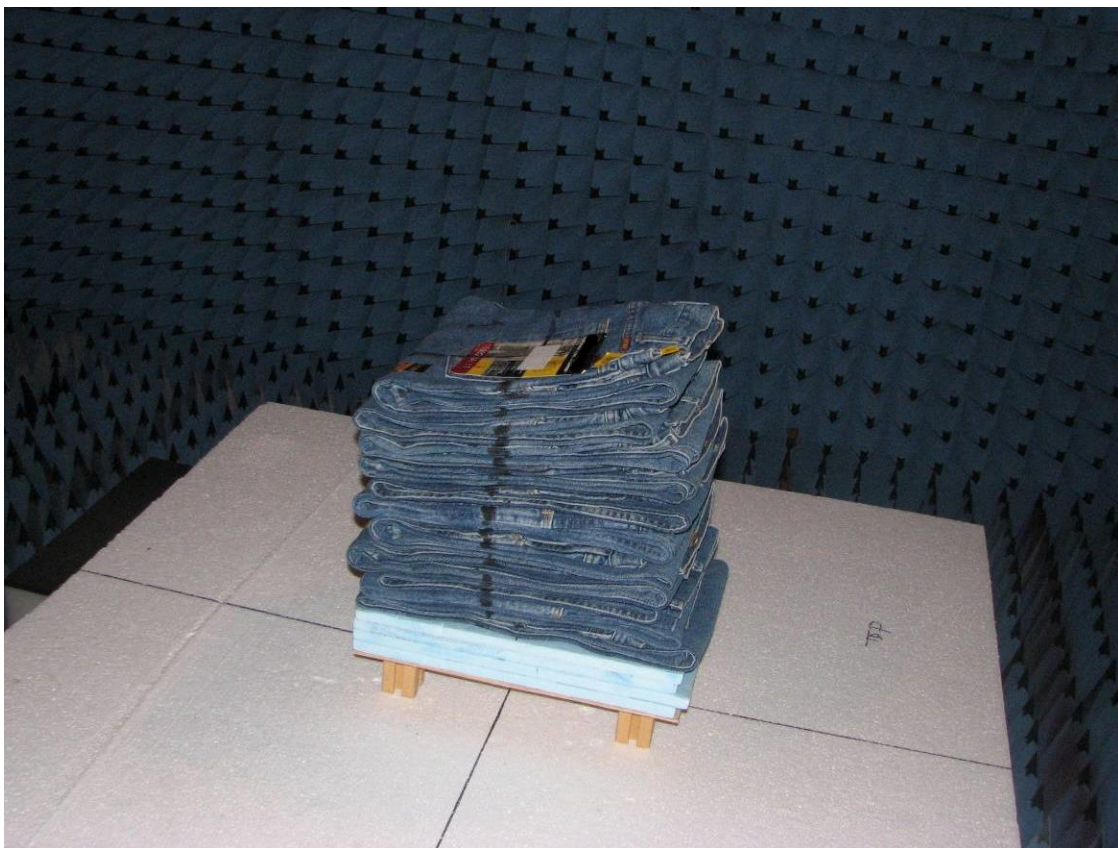
Figure 5: Multi Inlay Proximity Test with Denim
