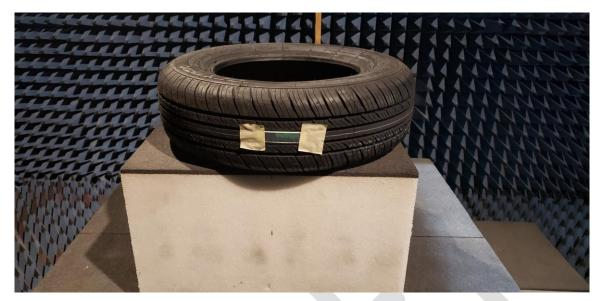
Figure 2: Position of Tag on Tire
