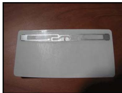
Photograph 8: RFID Standard Footprint Tag
